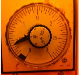
Ex. 90 sec exposure = "1.5" on the pointer and "1 m" on the multiplier
